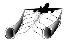
Wake vortices spread laterally away from the aircraft and descend approximately 500 to 900 feet at distances of up to five miles behind it. These vortices tend to descend at approximately 300 to 500 feet per minute during the first 30 seconds
